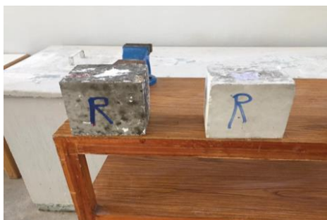
Figure 10: Comparison of specimen's color in different curing conditions. Left SRC specimen without water repellent cured in dead sea water, right specimen cured in plain water.
