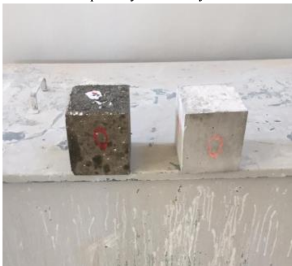
Figure 9: Comparison of specimen's color in different curing conditions. Left OPC specimen without water repellent cured in Dead Sea water, right same specimen cured in plain water.
