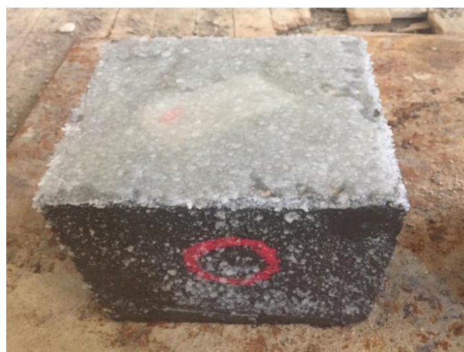
Figure 12: Salt crystallization on the surface of specimens cured in Dead Sea water
