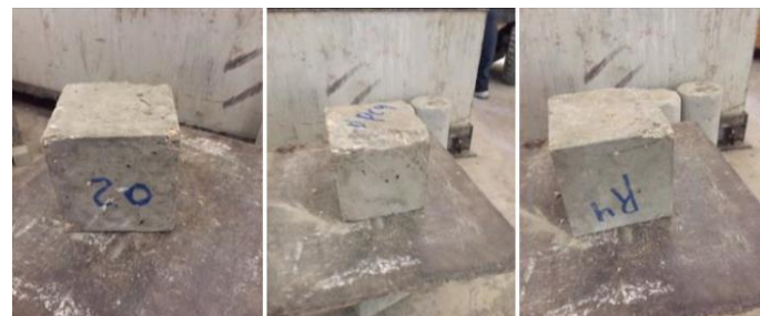
Figure 11: Specimens colour with water repellent cured in Dead Sea water. Left OPC sample, middle PPC sample, right SRC sample
