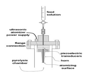
FIG. 2 System of Spray pyrolysis reactor system, showing feeding unit details and ultrasonic atomizer location in pyrolysis chamber [35].
