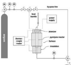
FIG. 1 System of spray pyrolysis reactor and supportive equipment [35].
