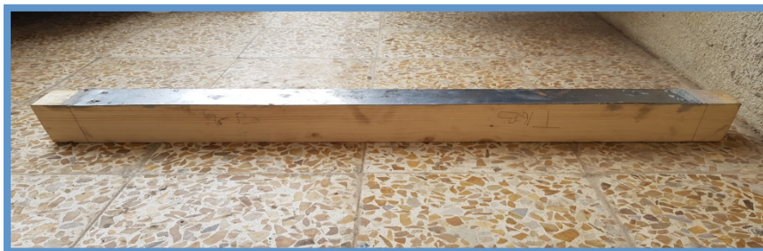
10. Beam strengthened by steel plate.
