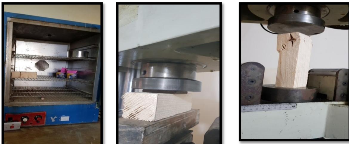
Fig. 1. Mechanical properties tests of timber specimens
