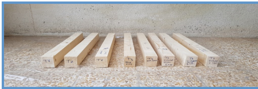
1. Specimens of beams before strengthening.
