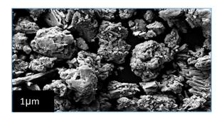
Fig. 1 Electron photographs of CdS nanoparticle(SEM).
