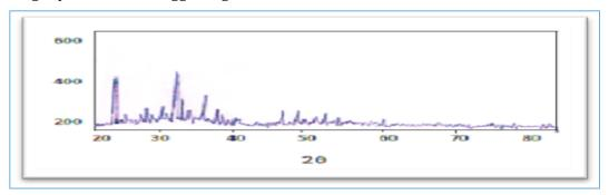
Fig. 3 The XRD pattern of CdS nanostructure obtained from sol-gel process
