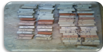
Figure 8: (G5, B5, P5) Modulus of rupture for prisms for different ages for the addition of glass powder, brick powder and porcelain powder respectively. (i)Prisms after fracture
